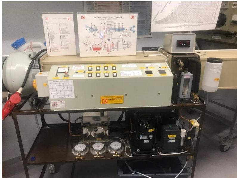
Figuur 5: De Hilton Air Conditioning Laboratory Unit
